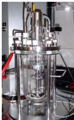
Stirred tank reactor
