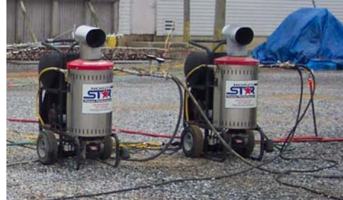
Example of Steam Generators
