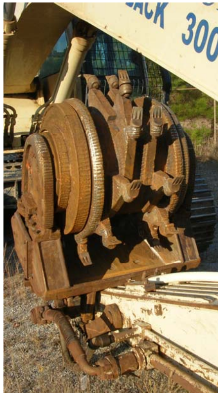
Figure 2: In-situ Blender with Specially Designed Teeth
