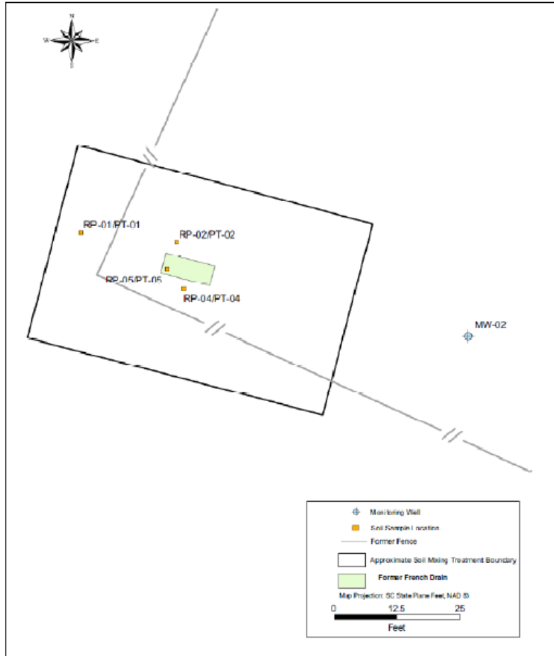
Figure 4: Post-treatment Soil Sample Locations
