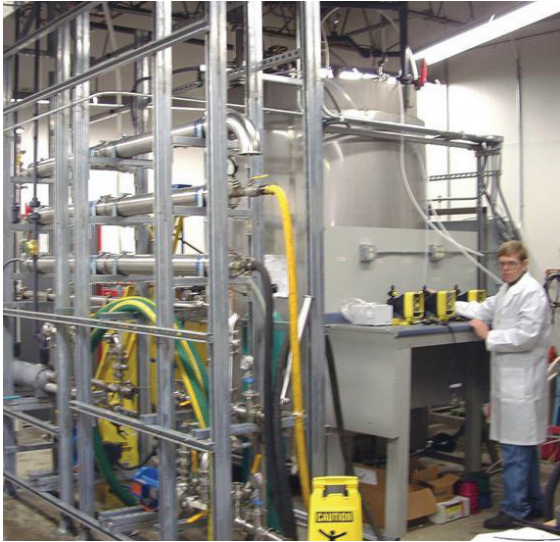
Shaw's 4000-L Fermentor and Cell Concentrator
